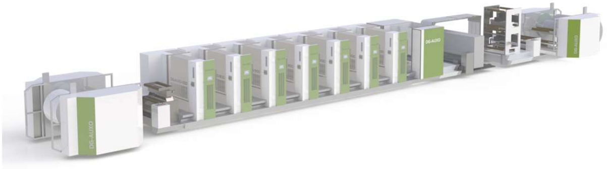
Figure 9 DG-AUXO 900 with 7 print units for ECG printing
